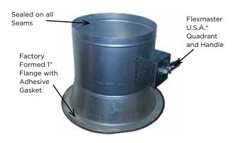
The Flexmaster U.S.A.® CBD-SOG-BO3 UT 3000G fitting is a factory sealed fitting, manufactured from 26 gauge, or heavier, galvanized steel to meet SMACNA and UMC Standards for commercial construction.
